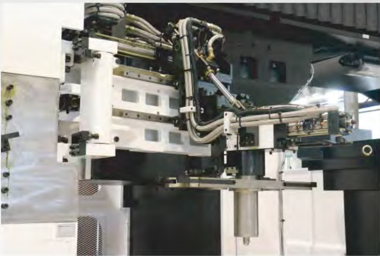
1. The vertical and horizontal tool magazine
