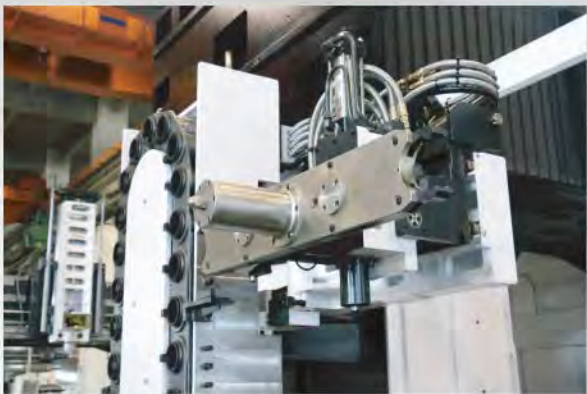
1. The vertical and horizontal tool magazine
