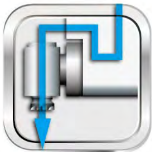
Angular head center coolant mechanism (UAC)
