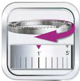
Angular head C-axis 1 degree positioning mechanism (TWC)
