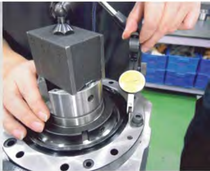
• End surface flatness correction
