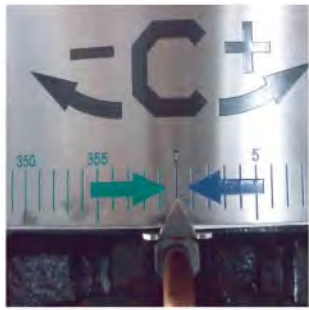
Minimum optional configuration A/C-axis positioning indexing: 1 degree
