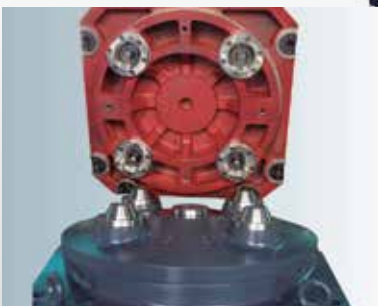
Clamping a pallet using 4 cones in the pallet corners is guaranty for a perfect gripping force of 35,5 kN //
